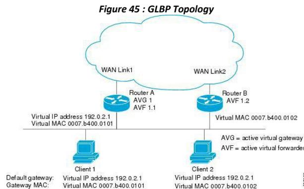
If router A becomes unavailable, client 1 does not lose access to the WAN because router B assumes responsibility for forwarding packets sent to the virtual MAC address of router A and for responding to packets sent to its own virtual MAC address. Router B also assumes the role of the AVG for the entire GLBP group. Communication for the GLBP members continues despite the failure of a router in the GLBP group.
