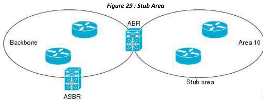
Stub areas use a default route for all traffic that needs to go through the backbone area to the external autonomous system. The default route is an Inter-Area-Prefix LSA with the prefix length set to 0 for IPv6.
