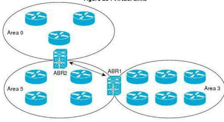
You can also use virtual links to temporarily recover from a partitioned area, which occurs when a link within the area fails, isolating part of the area from reaching the designated ABR to the backbone area.
