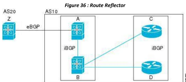
The route reflector and its client peers form a cluster. You do not have to configure all iBGP peers to act as client peers of the route reflector. You must configure any nonclient peer as fully meshed to guarantee that complete BGP updates reach all peers.
