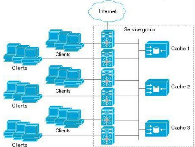
You can configure a service group as open or closed. An open service group forwards traffic without redirection if there is no cache engine to redirect the traffic to. A closed service group drops traffic if there is no cache engine to redirect the traffic to.
