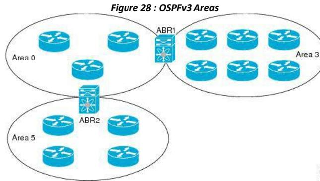
The ABR has a separate link-state database for each area which it connects to. The ABR sends Inter-Area Prefix (type 3) LSAs from one connected area to the backbone area. The backbone area sends summarized information about one area to another area. In the figure, Area 0 sends summarized information about Area 5 to Area 3.
