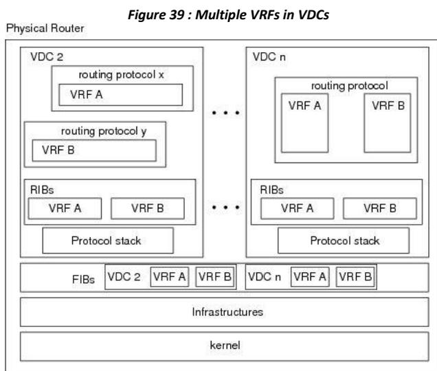
A VRF name is local to a VDC, so you can configure two VRFs with the same name if the VRFs exist in different VDCs. In Figure 14-1, VRF A in VDC 2 is independent of VRF B and VRF A in VDC n.
