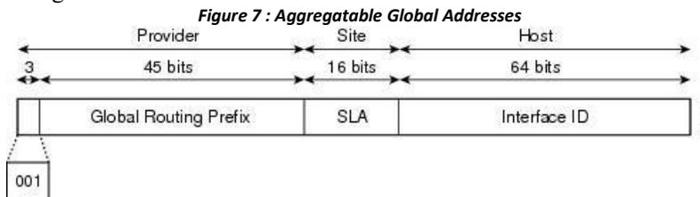
Addresses with a prefix of 2000::/3 (001) through E000::/3 (111) are required to have 64-bit interface identifiers in the extended universal identifier (EUI)-64 format. The Internet Assigned Numbers Authority (IANA) allocates the IPv6 address space in the range of 2000::/16 to regional registries.
