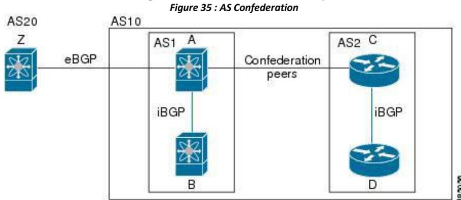
In this example, AS10 is split into two subautonomous systems, AS1 and AS2. Each subautonomous system is fully meshed, but there is only one link between the subautonomous systems. By using AS confederations, you can reduce the number of links compared to the fully meshed autonomous system.
