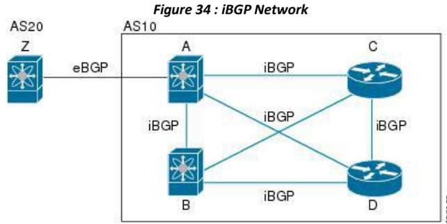
iBGP networks are fully meshed. Each iBGP peer has a direct connection to all other iBGP peers to prevent network loops.
