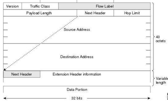
Optional extension headers and the data portion of the packet are after the eight fields of the base IPv6 packet header. If present, each extension header is aligned to 64 bits. There is no fixed number of extension headers in an IPv6 packet. Each extension header is identified by the Next Header field of the previous header.
