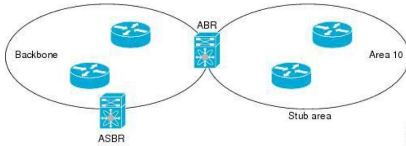
Stub areas use a default route for all traffic that needs to go through the backbone area to the external autonomous system. The default route is 0.0.0.0 for IPv4.
