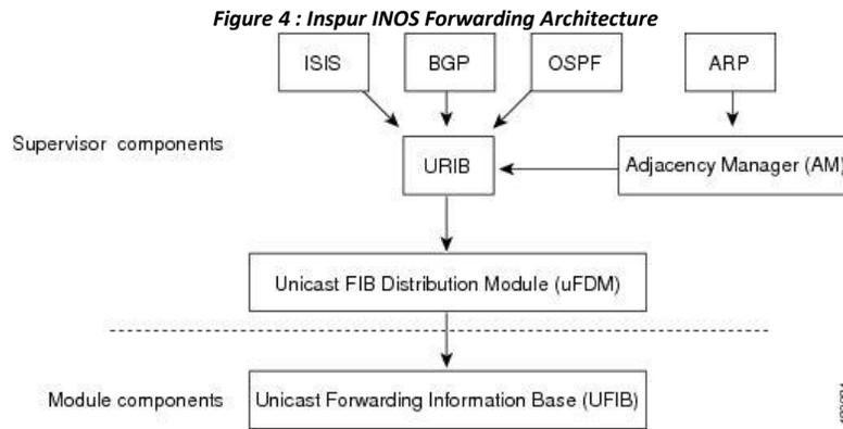
The unicast RIB exists on the active supervisor. It maintains the routing table with directly connected routes, static routes, and routes learned from dynamic unicast routing protocols. The unicast RIB also collects adjacency information from sources such as the Address Resolution Protocol (ARP). The unicast RIB determines the best next hop for a given route and populates the unicast forwarding information base (FIB) by using the services of the unicast FIB distribution module (FDM).
