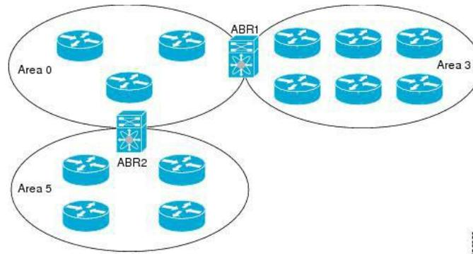
The ABR has a separate link-state database for each area to which it connects. The ABR sends Network Summary (type 3) from one connected area to the backbone area. The backbone area sends summarized information about one area to another area. In the OSPFv2 Areas Figure, Area 0 sends summarized information about Area 5 to Area 3.
