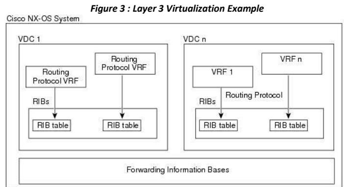
A VRF represents a Layer 3 addressing domain. Each Layer 3 interface (logical or physical) belongs to one VRF. A VRF belongs to one VDC. Each VDC can support multiple VRFs.
